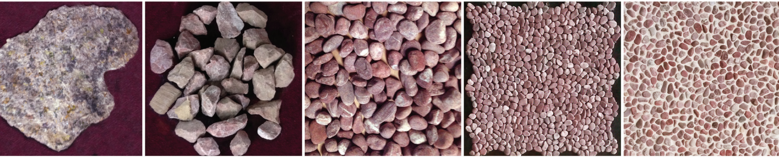
Above: left to right: A piece of the historic church's granite; the newly sourced granite gravel; the tumbled pebbles; the pebbles applied to the adhesive fabric; the fabric after mortar application.
